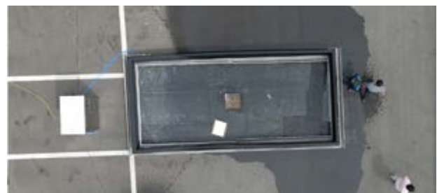
4. Fire release position fully submerged, battery stabilized
